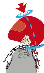
COUPLED AXIAL LOADING: Helps prevent axial loading only when the axial forces act in combination with other mechanisms.
