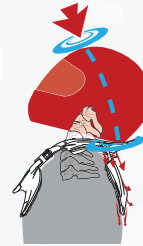
COUPLED AXIAL LOADING: Helps prevent axial loading only when the axial forces act in combination with other mechanisms.
